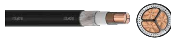
POLYCAB BS 6724 MC SWA LSZH (SHAPED CONDUCTOR) - Power Cable, 1.9/3.3 KV AC
